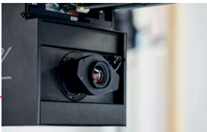
Camera system with a CMOS-based line sensor
